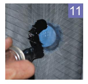
Apply a coat of Inner Liner Sealer around the outside edge of the patch to cover any excess buffing. This will ensure any buffed liner remains air-tight.
