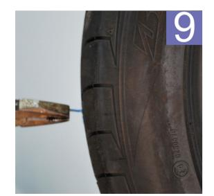
Pull the insert needle of the Mini Combi towards the outside of the tyre using pliers until the patch has seated on the cemented area.
