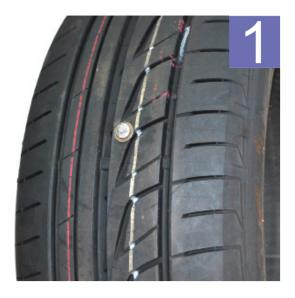
Locate the injury. It should be within the edges of the stabilliser belt on the crown or tread area of the tyre.
